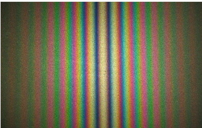
Figure 4. Fringe pattern produced with a Michelson interferometer using white light. As configured here, the central fringe is white rather than black [5].
