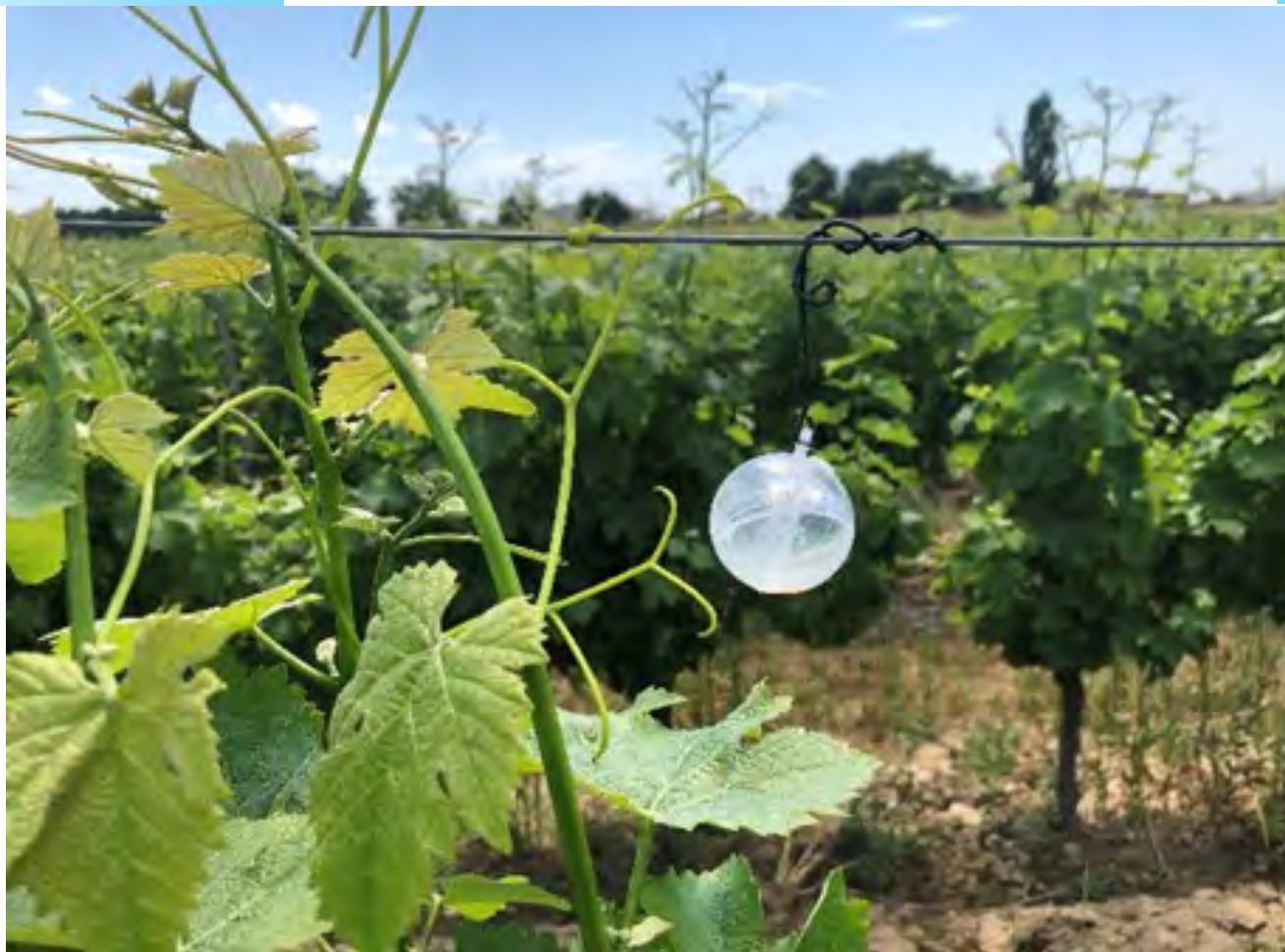
Figure 4. Ball with two GaNSes deployed in the field.
