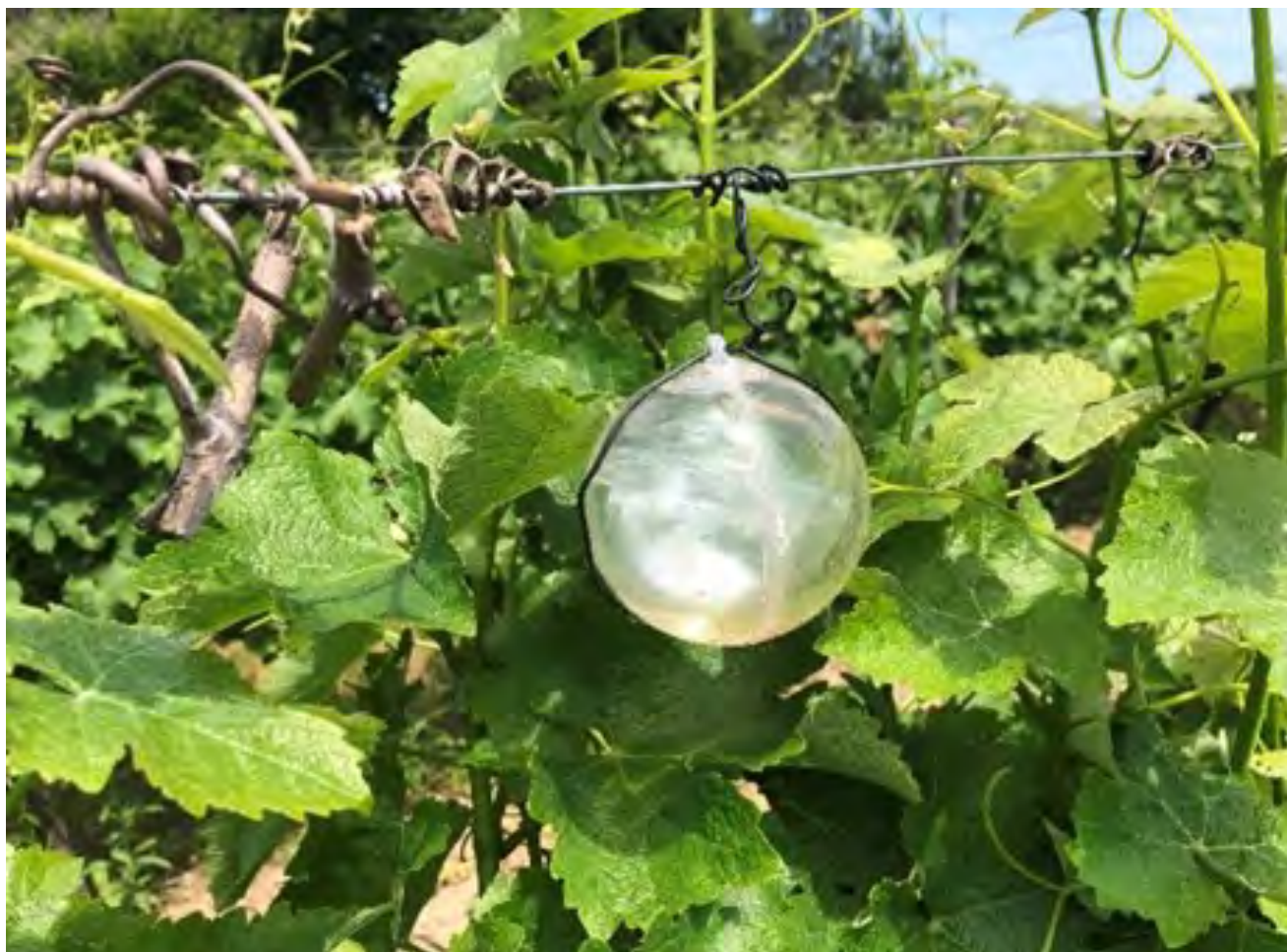
Figure 5. Ball with three GaNSes deployed in the field.
