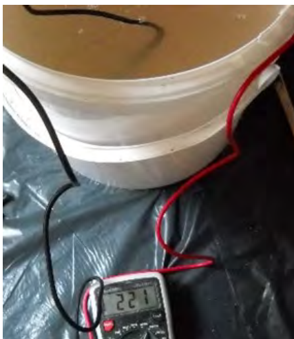
Figure 5. The voltage measured between the nano-coated copper plate and the platinum.
